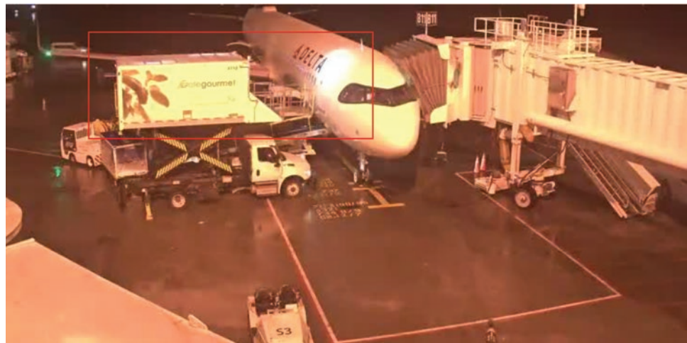
Figure 9 Congestion in case of bag loading and catering loading at the front of the aircraft
